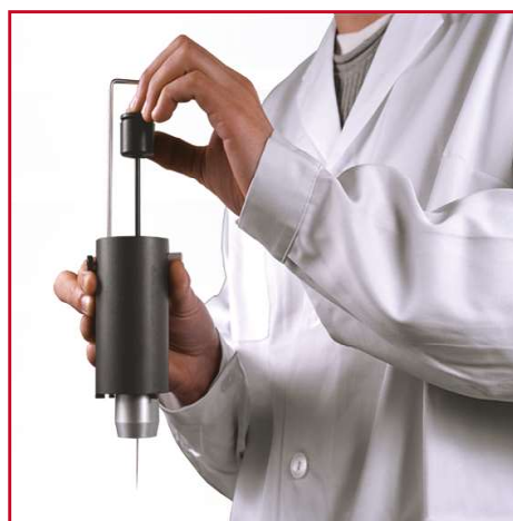
Inject the sample into the GC. Repeat this sequence for the additional samples.
